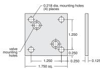
**Construction:** Black anodized finish, two mounting screws furnished.
